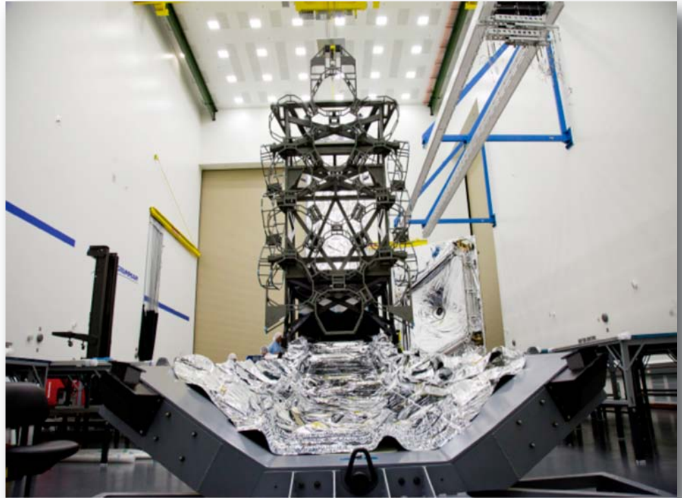
Figure 6: A view of the IVA showing the fore-sunshield palette, with membranes folded and stowed. The IVA also features a mockup of the primary mirror backplane, the skeleton structure which is used to assess envelope clearances during deployment testing.
