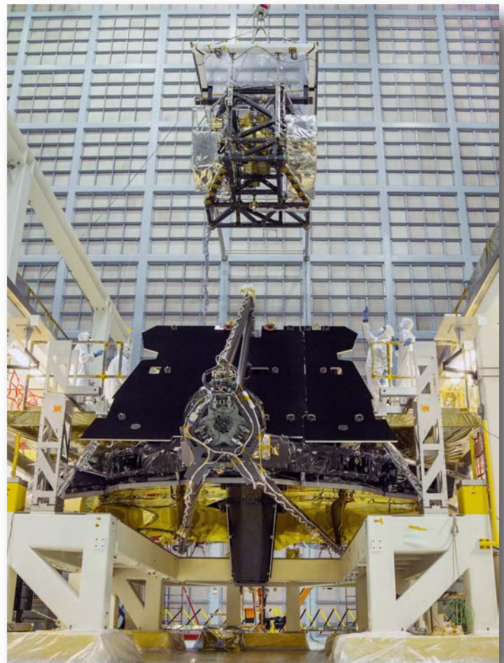
Figure 4. The JWST science instruments are lowered into position using a crane. The primary mirror segments can be seen facing the floor for this installation. A video of the installation process can be downloaded at http://svs.gsfc.nasa.gov/12273 .
