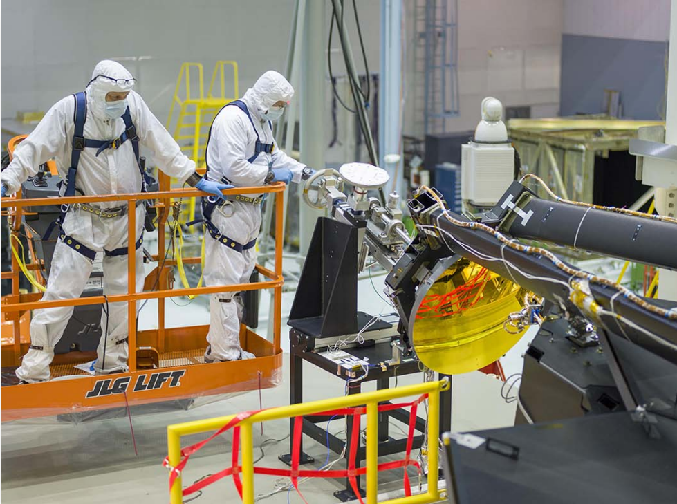
Figure 1. The secondary mirror was installed with the support structure in the stowed position. The process used a manual fixture situated down wind of the telescope in Goddard's cleanroom.
