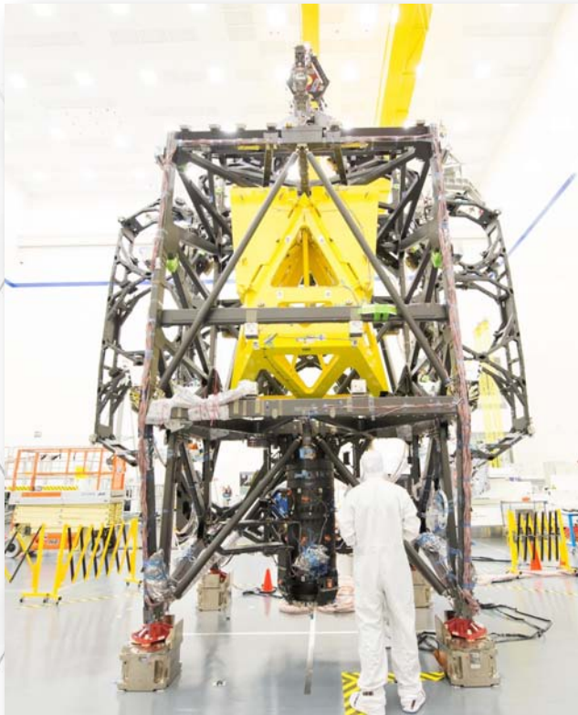
Figure 3: (below) Rear view of the JWST telescope structure showing the backplane support fixture (BSF). The yellow structure is a mass simulator for the Integrated Science Instrument Module (ISIM) which was installed for modal testing of the telescope structure. The stowed deployable tower assembly (DTA) is seen to the left of the standing figure. Credit: Northrop Grumman
