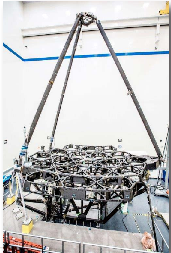
Figure 1: The JWST telescope structure in a clean room at Northrop Grumman, showing the fully deployed secondary mirror structure and the deployed primary mirror backplane wings. Credit: Northrop Grumman
