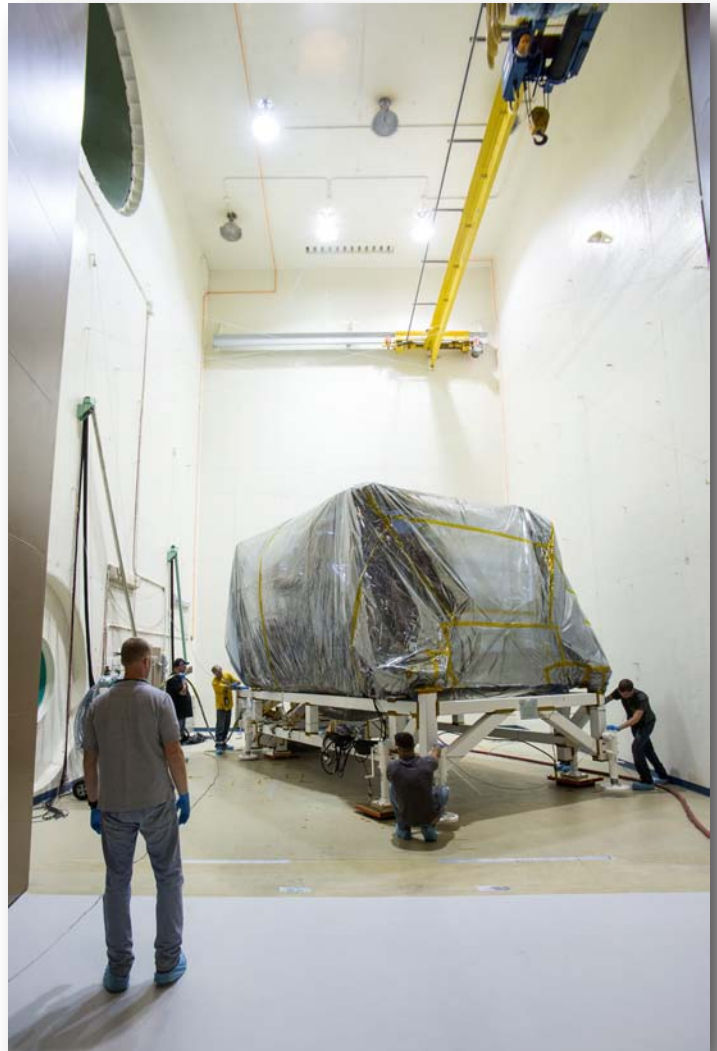
Figure 3: The acoustic test facility at Goddard Space Flight Center, where the ISIM will undergo testing later this summer. Note the huge feed horns that reproduce the acoustic environment of a rocket launch. Credit NASA/Chris Gunn
