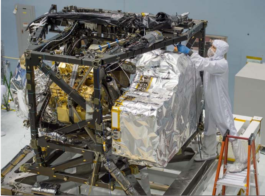
Figure 1: The ISIM structure and flight instruments, re-integrated and ready for environmental testing. Credit: NASA/Chris Gunn
