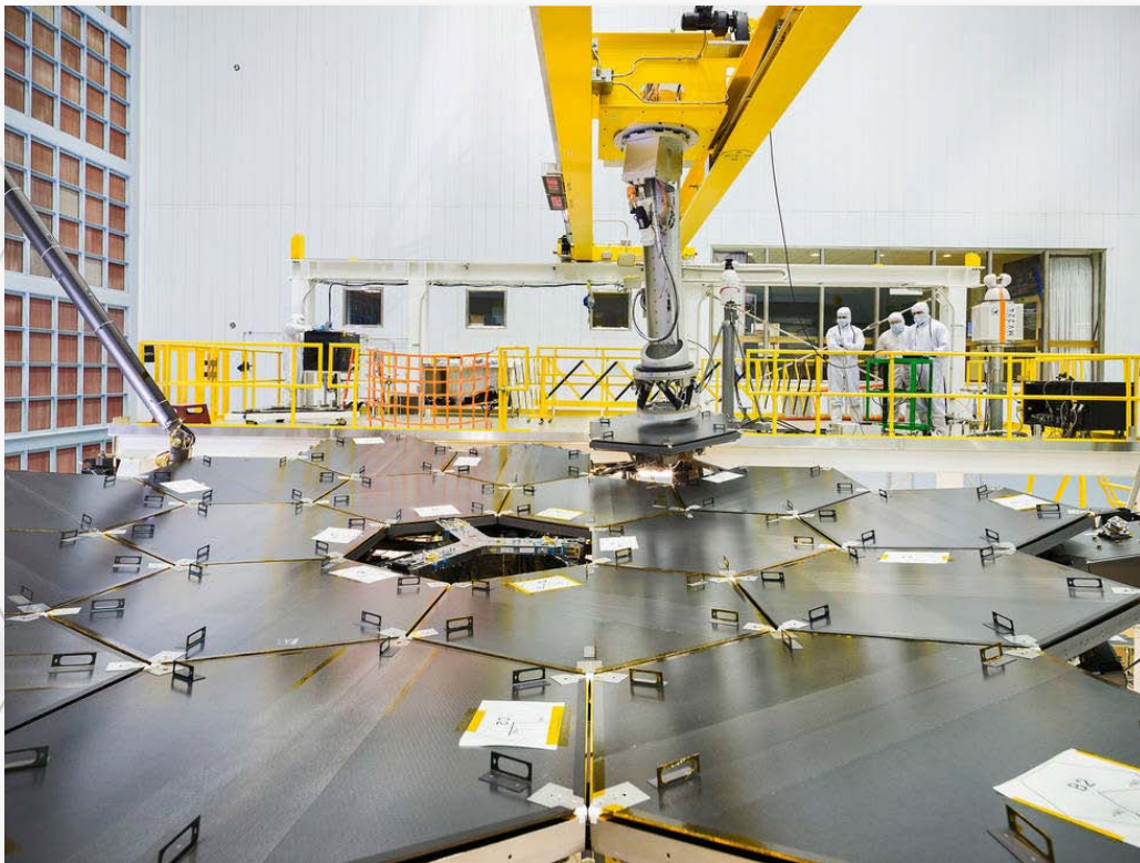
The 18th and final James Webb Space Telescope primary mirror segment is installed at NASA Goddard. Credit: NASA/Chris Gunn
