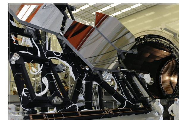
Three mirror segments about to undergo cryogenic testing at Marshall Space Flight Center. (Ball Aerospace)
